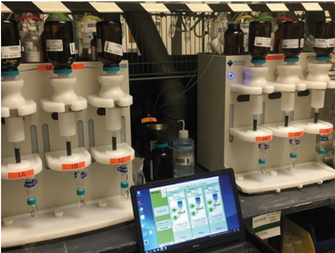
Figure 1. Two Biotage® Horizon 5000 extractors equipped with carbon cartridges for extraction. Both extractors are controlled using the PC in the middle of the image.
